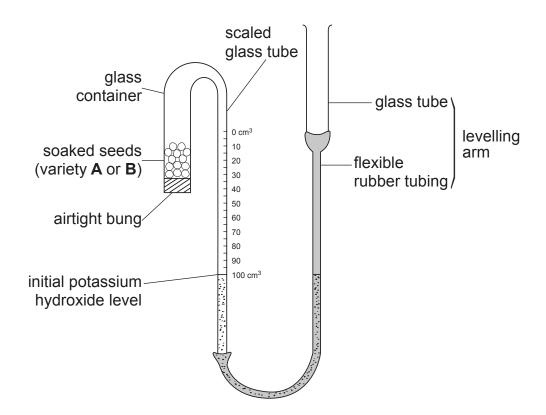
For each variety, 10 g of soaked peas were placed in the glass container with an airtight bung. The level of potassium hydroxide was adjusted to 100 cm<sup>3</sup> on the scale by raising or lowering the levelling arm.
